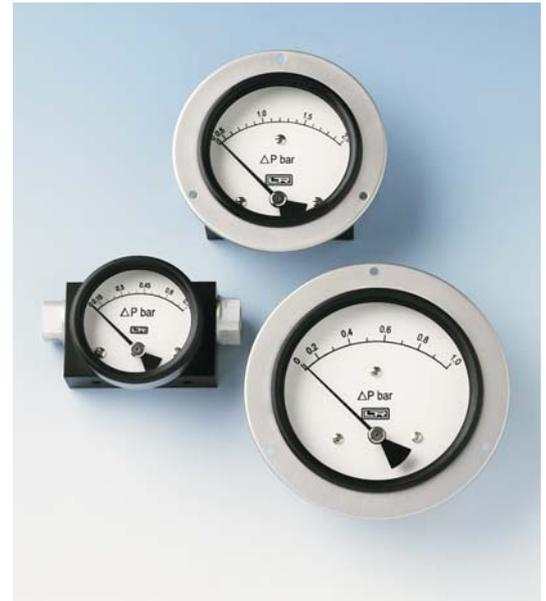
Piston type differential pressure gauge is mainly used for liquid application and where small migration between high and low input is permissible. It is recommended to monitor differential pressures on cartridge filters, pipeline systems, valves, pumps, brand flows, condensers of those media without any magnetic substances.
