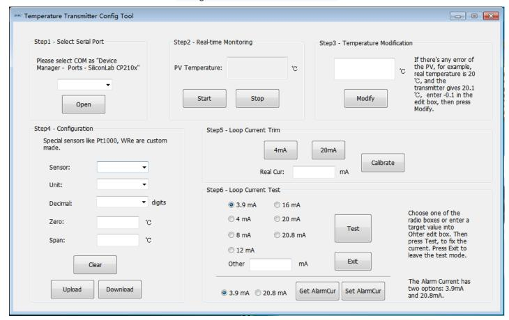
**Step 5** is Loop current trim. Select 4 mA or 20 mA and connect a standard ammeter with 24V circuit in series. 4 mA or 20 mA current calibration can be completed by entering the actual current value which displayed on the standard ammeter into Real Cur and clicking Calibrate.
