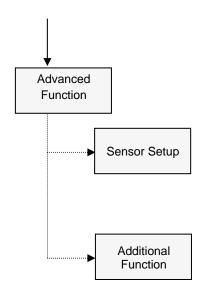
Set up sensor type, RTD connection, TC cold junction compensation and sensor upper / lower limit.
