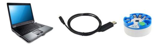
If ALIA software and driver are installed, connect temperature transmitter and computer with USB cable, and supply 24 VDC to temperature transmitter. Upon opening the software, select the correct comport in option **Step 1** and click OPEN.
