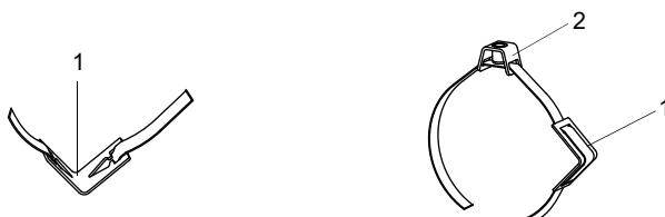
Fig. 6.40: Tension strap with metal spring and clamp
